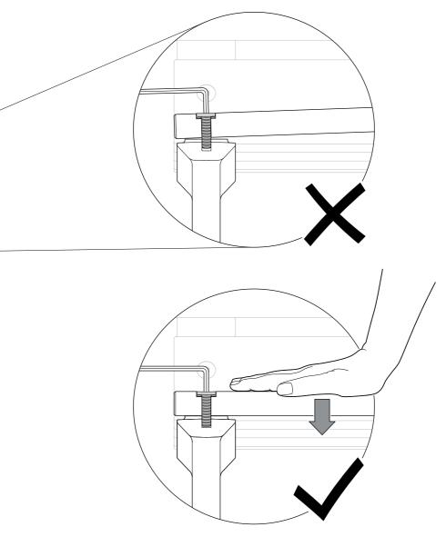
Apply an even and steady pressure on the center of the slats when tightening the screws.
